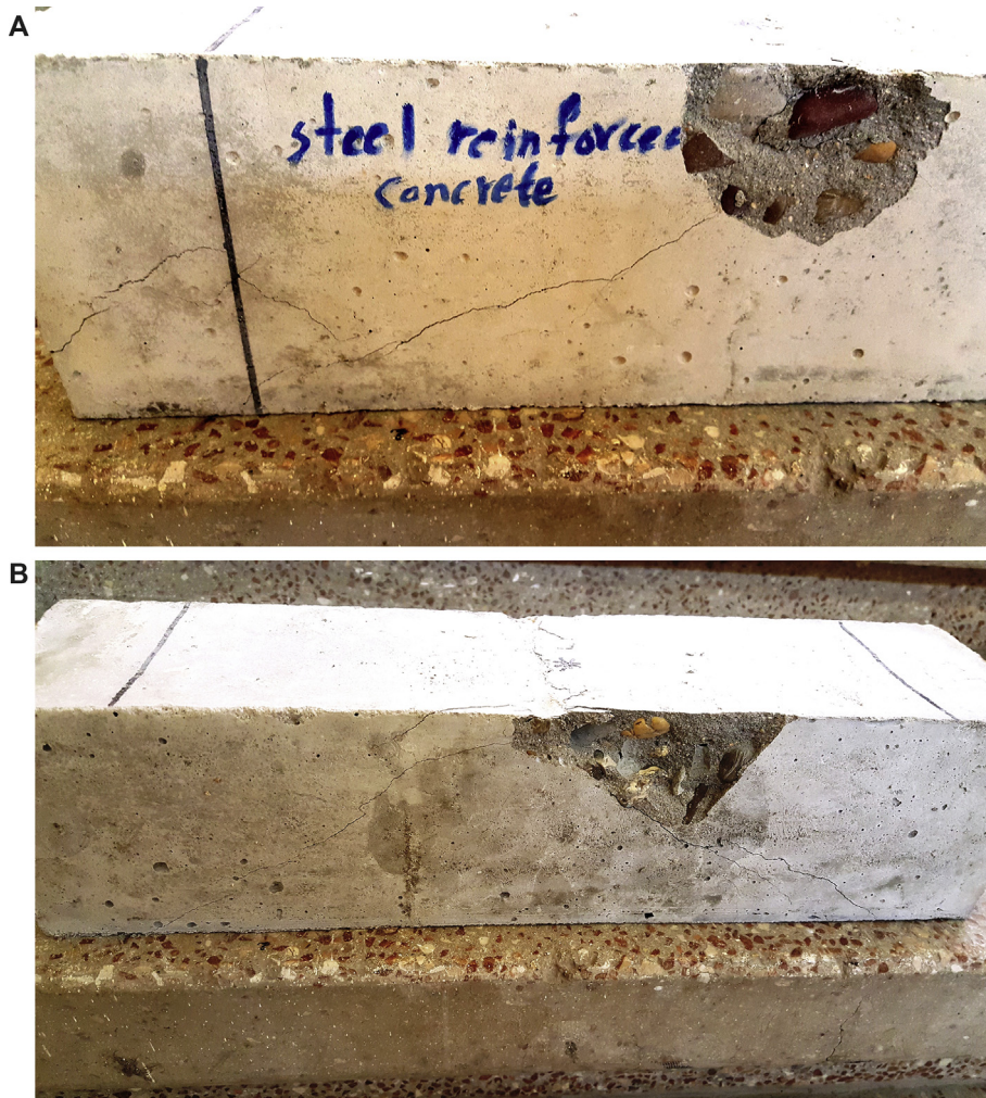
Fig. 11. (A, B): typical fracture of steel RC.
