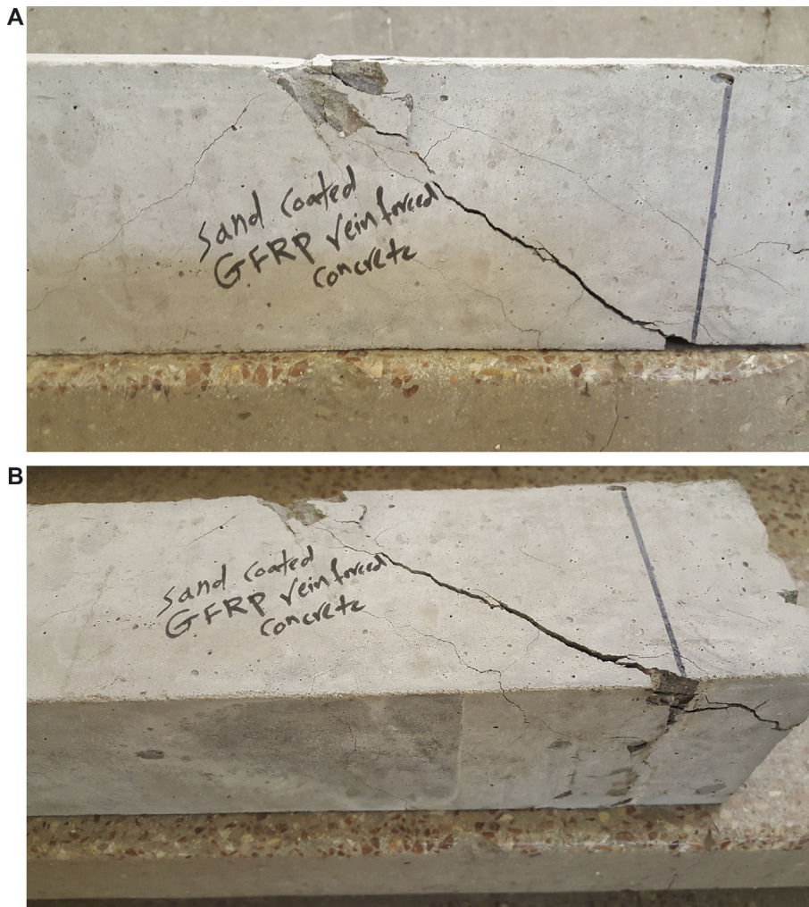
Fig. 10. (A, B): typical fracture of sand coated GFRP RC.
