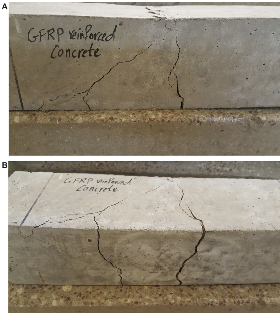
Fig. 9. (A, B): typical fracture of smooth GFRP RC.
